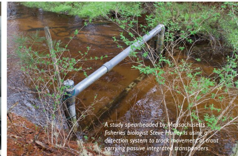
A study spearheaded by Massachusetts fisheries biologist Steve Hurley is using a detection system to track movement of trout carrying passive integrated transponders.
